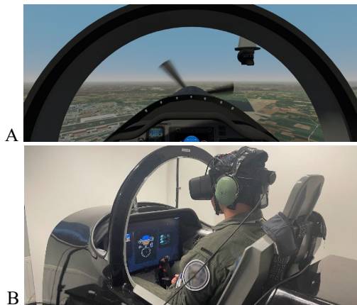
Fig. 1. Experimental set-up. A) Image taken from the simulated (VR) environment. B) Participants conducted the experimental tasks while seated in a PC-7 cockpit mock-up, wearing the VR-headset and EEG equipment.
