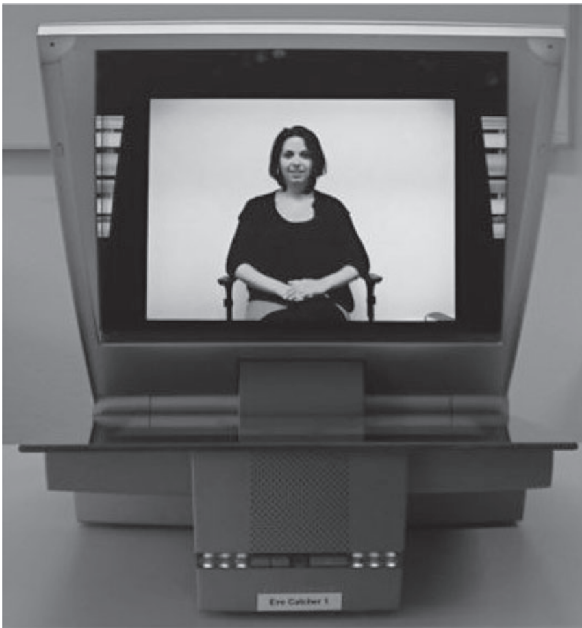
Figure 6 The Eye-Catcher seen from the front, with a video-image of the addressee
