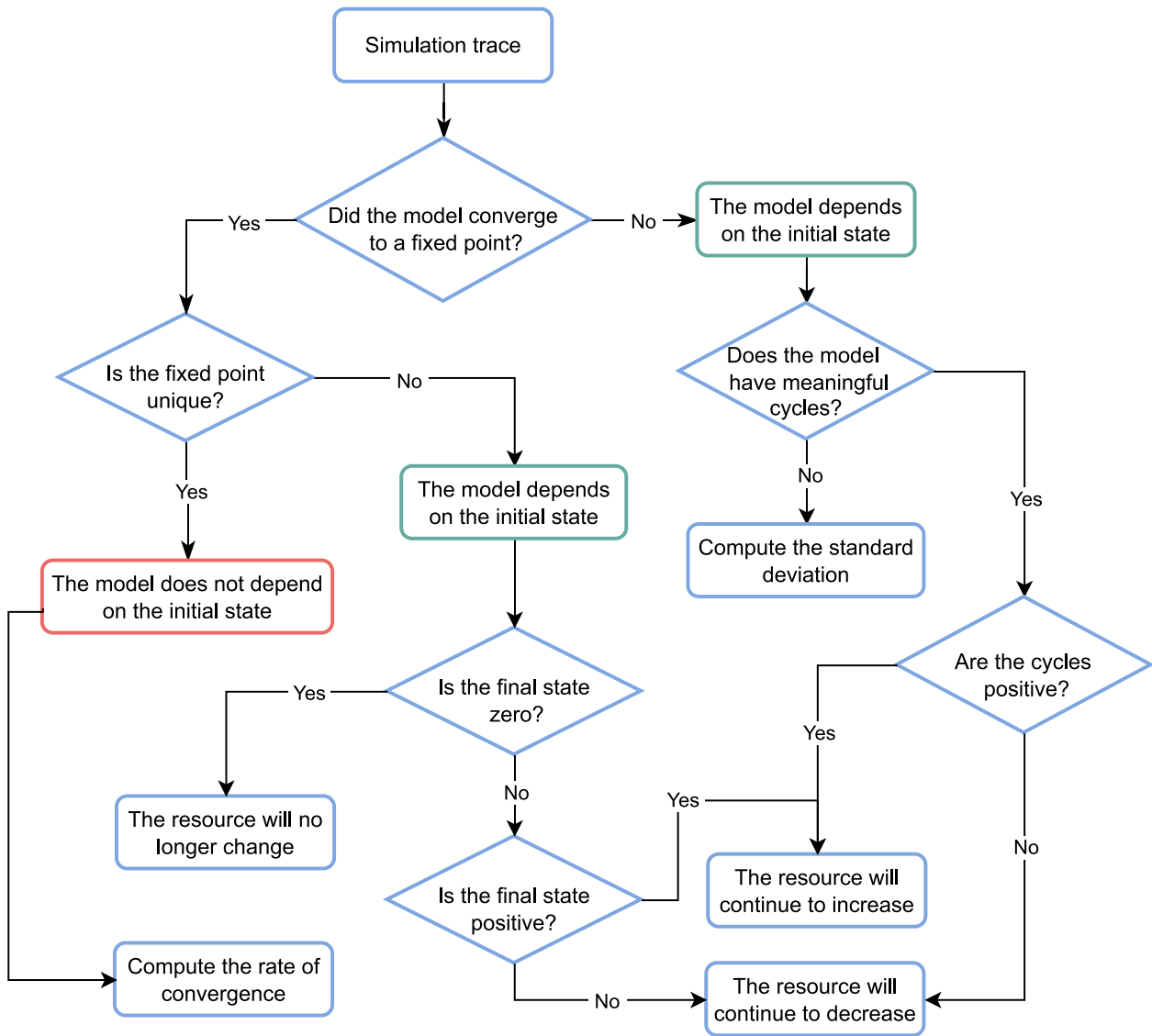
Fig. 6. Flow diagram indicating how to interpret the simulation results and different convergence behaviors.
